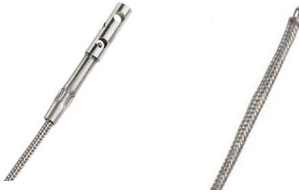
Figure B.6. Omega k-type thermocouples (type XCIB) used in USF's packed bed system.
